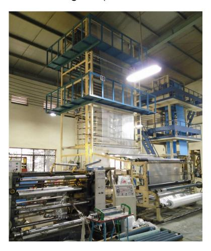
• PE shrink film blowing machine, auto – stick and protecting PE layer (4 layers):
