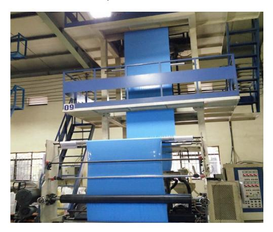
• PE blowing machine, Shrink film machine:
