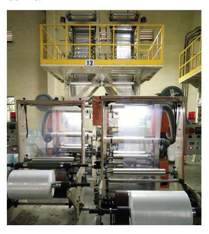
• PE Shrink Film Machine for big size (maximum diameter 2.5m):
